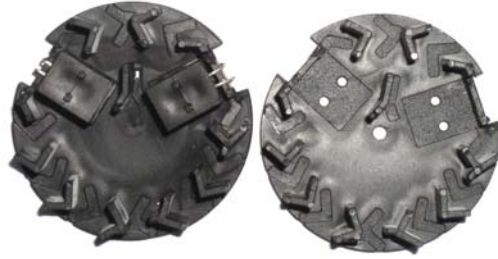
Figure 10. Internal Construction of Smoke Chamber
