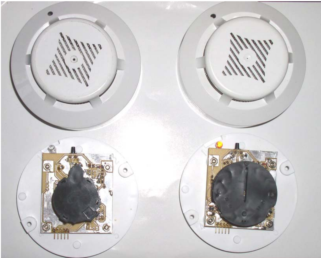
Figure 11. Two Detectors with Different Chamber Sizes and Different Chamber LED and Photodiodes
