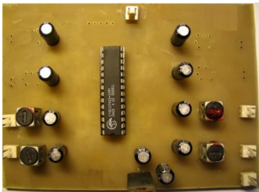
Figure 13. Parking Assistant Slave Device Top Side
